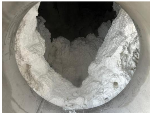
Figure 3 Condition after mechanical cleaning & steam condensate flow (Before Startup)
